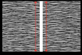
Ebbtide shown with recommended random match trin lines. For best installation, double cutting on the wall is recommended. The horizonta design elements will create an obvious and natural ioin at the seam.
