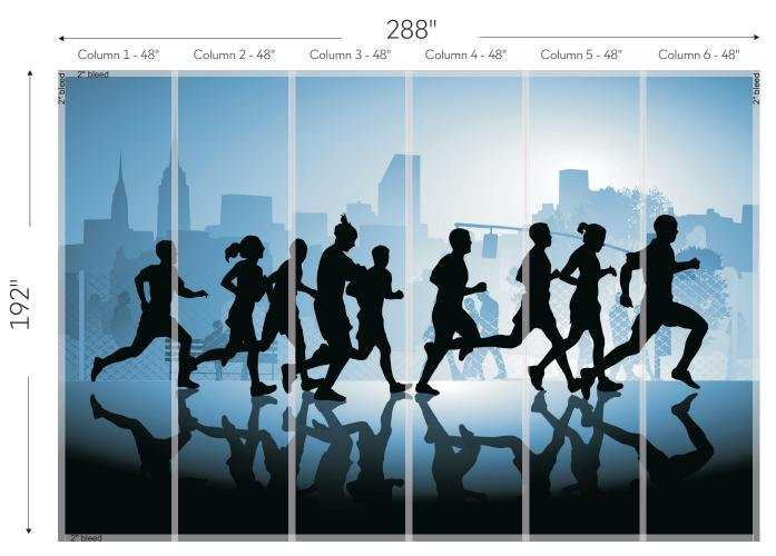
A 2 inch overlap is printed at all seams. Each adjacent panel is printed in the opposite direction to manage shading. Image is printed with 2" bleed on each edge
