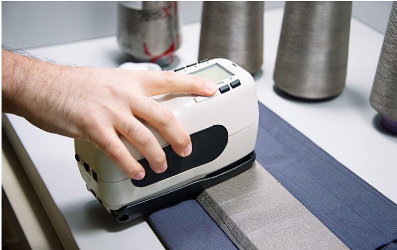
Yarn from multiple cones are knitted into tubes so Noble can perform quality and compliance tests. A spectrophotometer is used to measure color consistency from cone to cone
